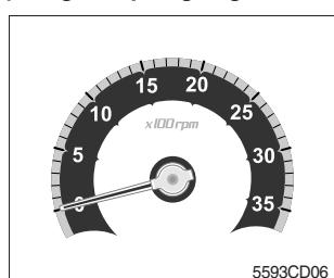
① This gauge displays the number of engine revolutions per minute.
